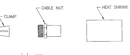
1. Place heat shrink and cable nut over outer jacket of cable. Trim outer jacket to expose copper corrugate DO NOT NICK CORRUGATE! Cut corrugate and dielectric to dimensions shown and tin center conductor.
